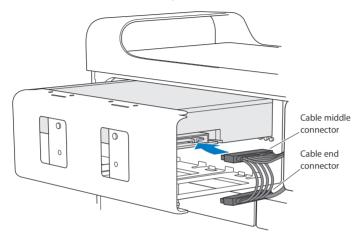
9 Lift the latch and then slide the carrier into the optical drive bay, pushing it into place.
