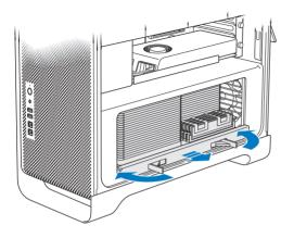
4 Remove the processor tray and lay it on a soft, clean cloth on the desk or work surface, to protect the tray and avoid scratching the work surface.
