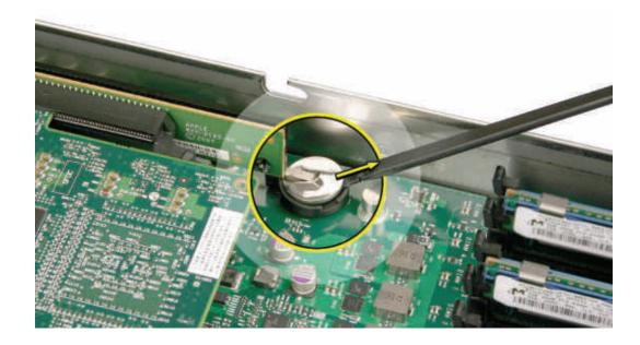
3. Insert the replacement battery in the holder with the positive side (+) up and the negative side down.
