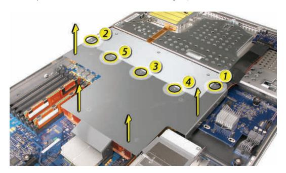
Caution: Try not to completely remove the screws from the airflow duct. Tiny black rubber washers hold these screws captive on the underside of the airflow duct. If the screws are completely removed, these washers can easily fall into the enclosure and become lost.
