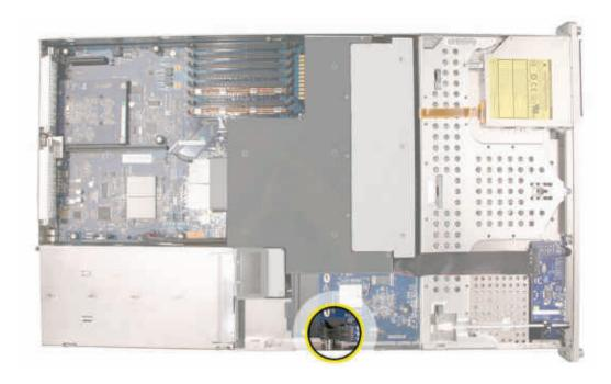
2. Disconnect the power distribution board cable from the drive interconnect backplane and the power distribution board. Remove the cable from the enclosure.
