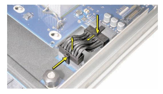
3. Release the two locking levers on the front panel board cable connector and disconnect the cable from the front panel board. Move the front panel board cable out of the way.
