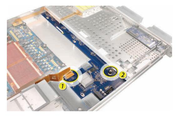
6. Shift the backplane to the left (towards the enclosure side), in the direction of the arrow shown, until it clears the four mushroom-shaped standoffs that hold the backplane in place.
