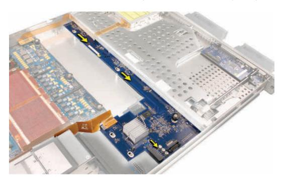
Rotate the backplane up slightly from the logic board side (as shown), and carefully pull the backplane up and toward the logic board to free it from the standoffs and four backplane alignment slots in the enclosure. Be careful not to let any backplane components come into contact with the standoffs or the enclosure as you remove the backplane.
