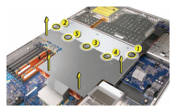
Caution: Try not to completely remove the screws from the airflow duct. Tiny black rubber washers hold these screws captive on the underside of the airflow duct. If the screws are completely removed, these washers can easily fall into the enclosure and become lost.
