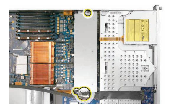
**Note:** You may encounter some resistance around the fan array power connector during removal. If so, carefully rotate the fan array as shown to disconnect it from the power distribution board below, and then lift the fan array out of the computer.
