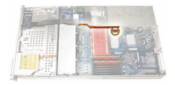
2. Disconnect the backplane-to-logic board cable from the drive interconnect backplane and remove the cable from the Xserve.
