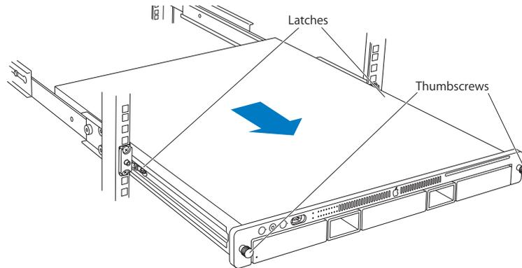
8. When the safety latches engage, grip the Xserve where it emerges from the rack, press down on the latch tabs with your thumbs, and slide the Xserve the rest of the way out of the rack.
