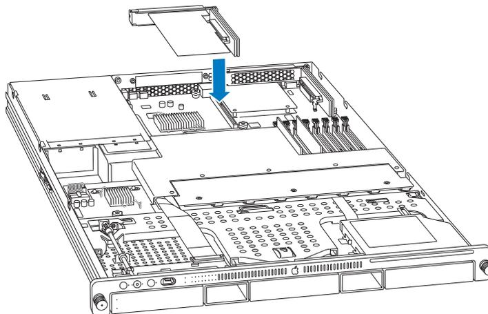
3. Tighten the captive screws that secure the riser bracket to the back panel.
