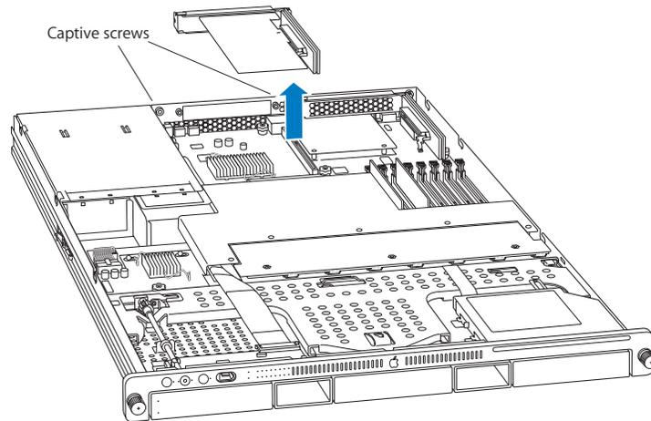
3. Tilt the expansion card up so that its port clears the enclosure, and remove the riser and card from the Xserve.
