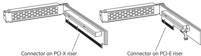
When replacing a riser card, you must transfer the installed PCI card to the replacement riser card.
